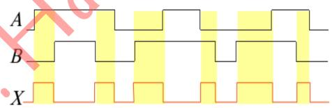
□ Notice that the XOR gate will produce a HIGH only when exactly one input is HIGH.
